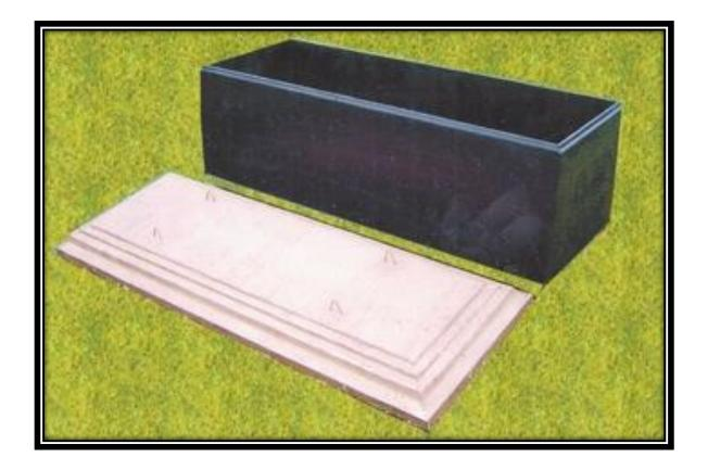
The Deluxe Vault has a tiered lid for more strength. The top is painted with black asphalt and has an option of a copper painted top. The box is coated with black asphalt paint and asphalt applied between the tongue and groove of the lid and box where joined.
